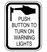
RRFB PUSHBUTTON SIGN (NOT TO SCALE)
