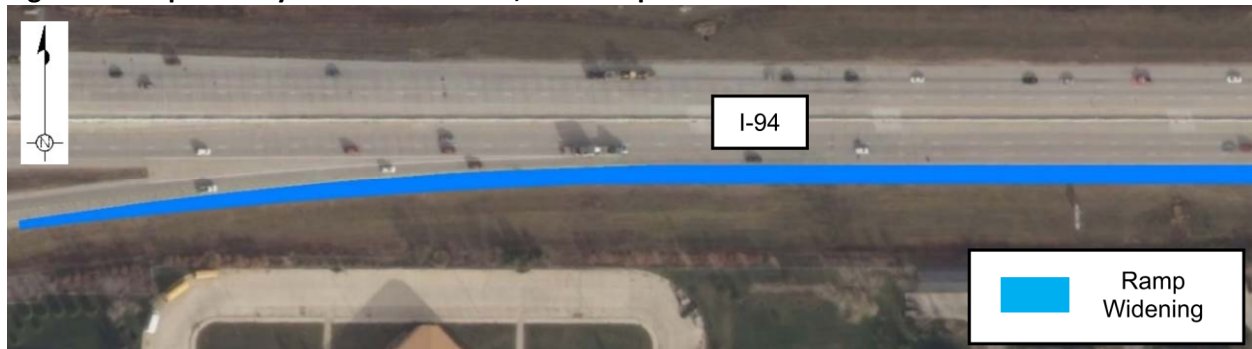
Figure 2 - Proposed Layout: Lane Addition, I-29 Ramp to I-94
