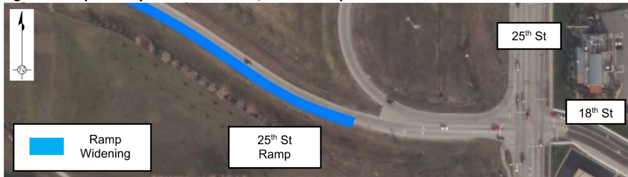
Figure 4 - Proposed Layout: Lane Addition, 25th St Ramp
