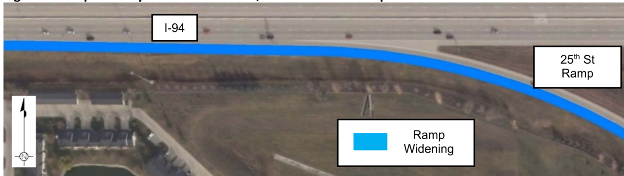
Figure 3 - Proposed Layout: Lane Addition, I-94 to 25th St Ramp
