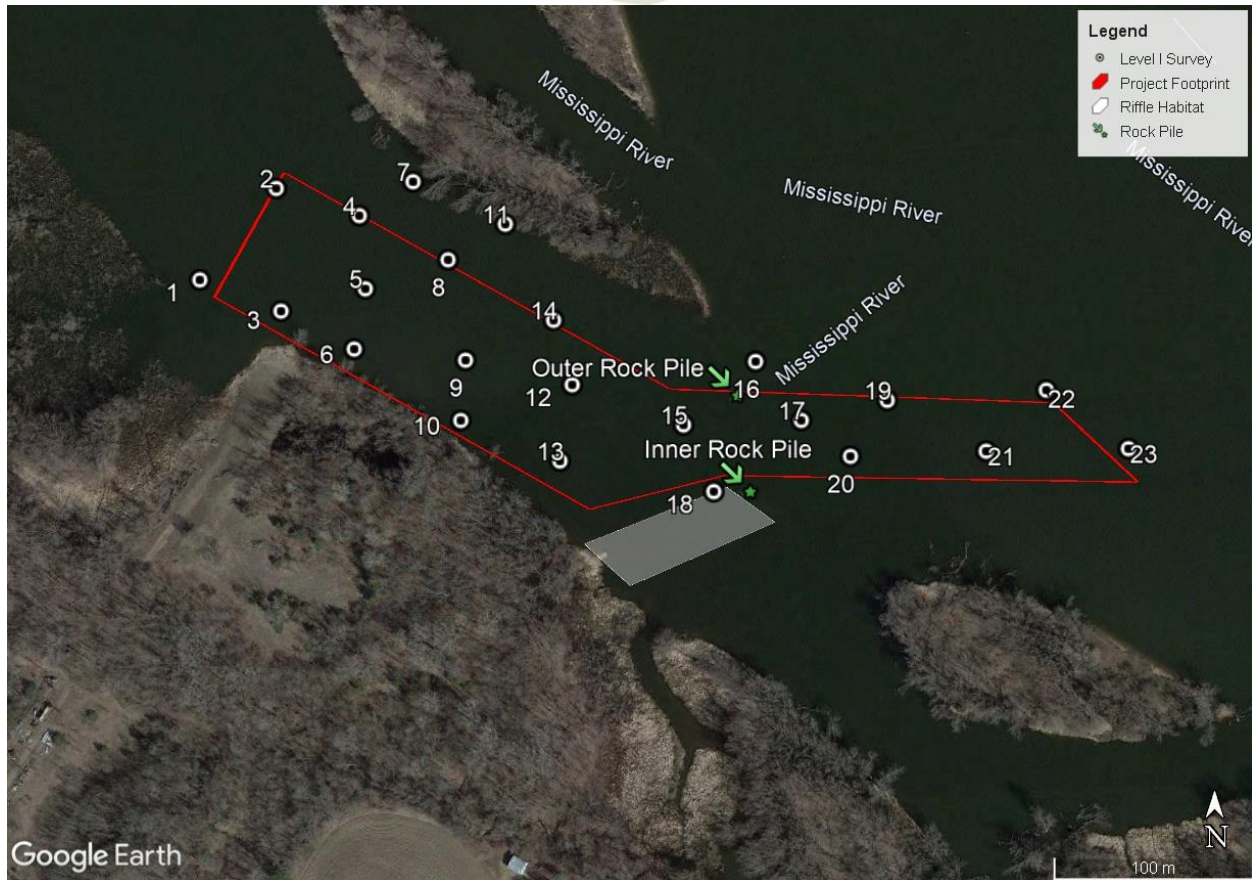
Figure 2. Aerial image of the project footprint and centroid of each Level I survey. The locations of the riffle and rock piles are shown.
